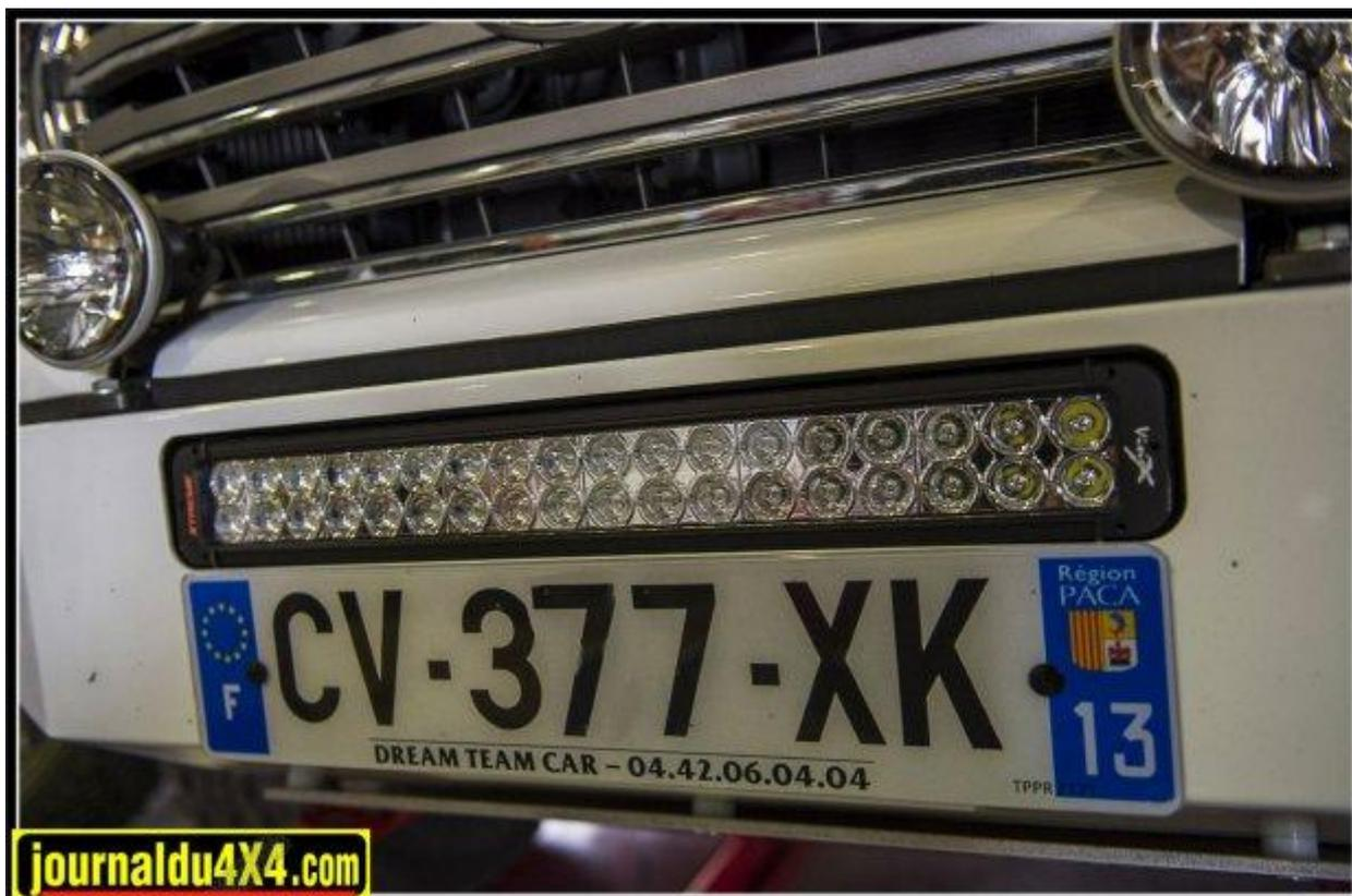
rampe de 36 LED Vision X XMITTER PRIME XP 36 LED 17.748 LM 180W
